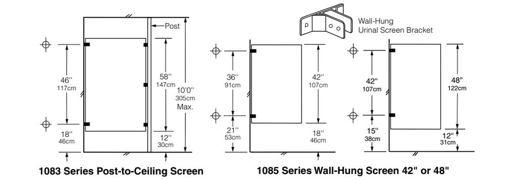
⊕ These mounting points require backing. For suggested backing methods, Bobrick Advisory Bulletins TB-32 for ceiling-hung installations and TB-46 for floor-anchored are available upon request.
